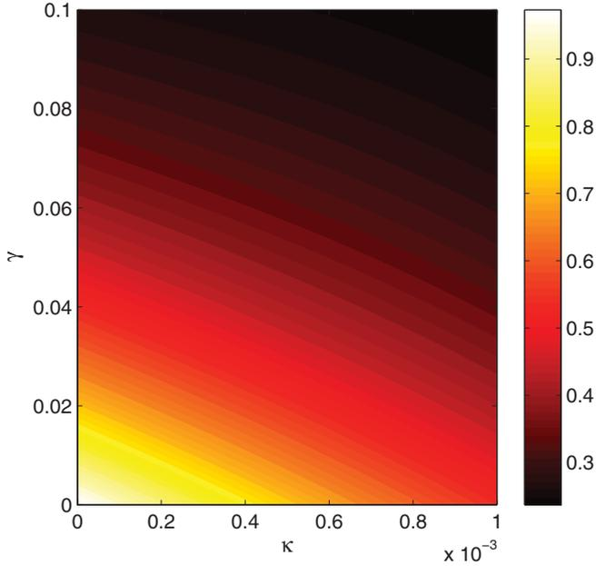
FIG. 7. (Color online) Contour plot of the final population  $\rho_{22}$  (at time  $t = 300/\delta$ ) for two-photon transfer as a function of atomic dissipation rate  $\gamma$  and cavity dissipation rate  $\kappa$  (both in units of  $\delta$ ).
