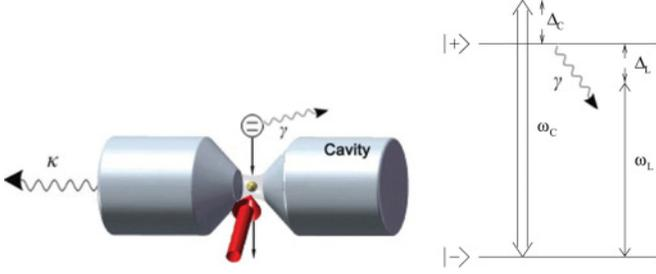
FIG. 1. (Color online) Configuration of the process: A two-level atom travels through a QED cavity and a transverse laser beam. The configuration is such that the cavity and laser fields partially overlap and the cavity field is crossed first by the atom [18].
