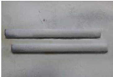
Figure 2.11 Powder tension samples covered with developer material
