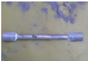
Figure 2.13 52.8% of wt. Ni-Ti tension sample applied to magnetic inspection
