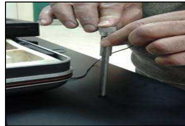
Figure 2.8 Fatigue sample inspection using ultrasonic method
