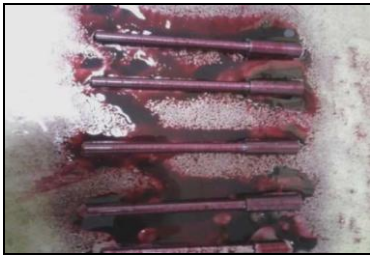
Figure 2.5 Applying die penetrant to fatigue samples
