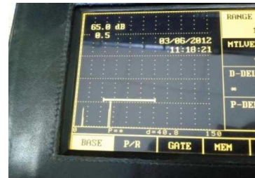
Figure 2.14 Edge reflections for fatigue sample inspected by ultrasonic waves showed on the digital screen
