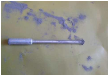
Figure 2.12 50% of wt. Ni-Ti fatigue sample applied to magnetic inspection
