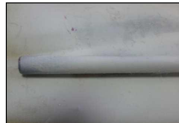
Figure 2.9 50% of wt. Ni-Ti fatigue sample covered with developer showed no surface defects
