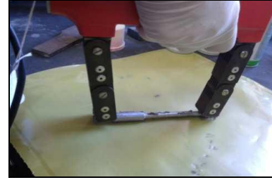
Figure 2.7 Fatigue sample magnetized by means of prods
