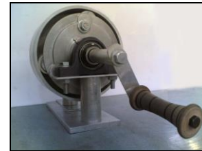
Fig. 1. The fabricated speed reducer after assembled
