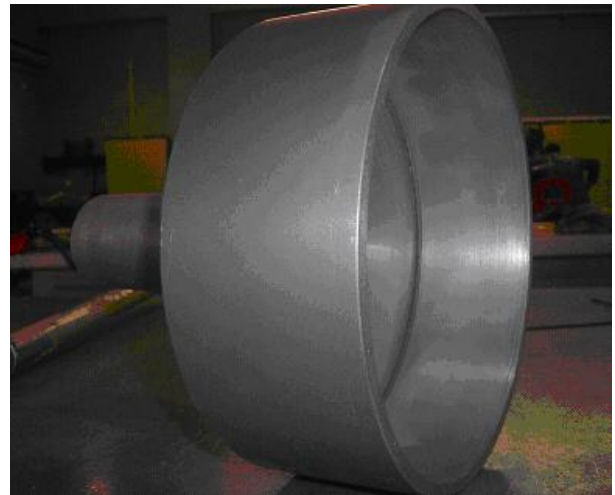
Figure 10: Casted Output Member
