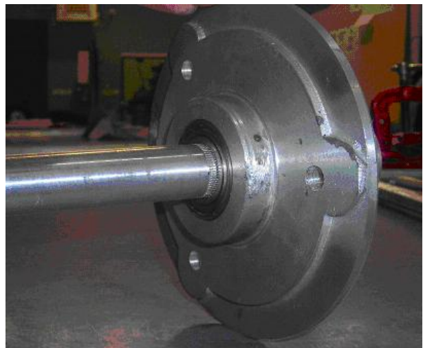
Figure 11: Casted midplate and input member
