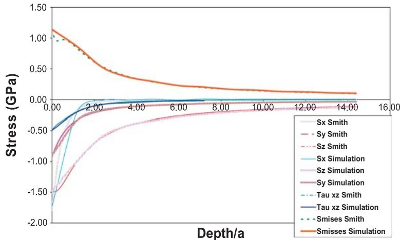
Figure 3. Smith proof for identical solid roller model under combined loading
