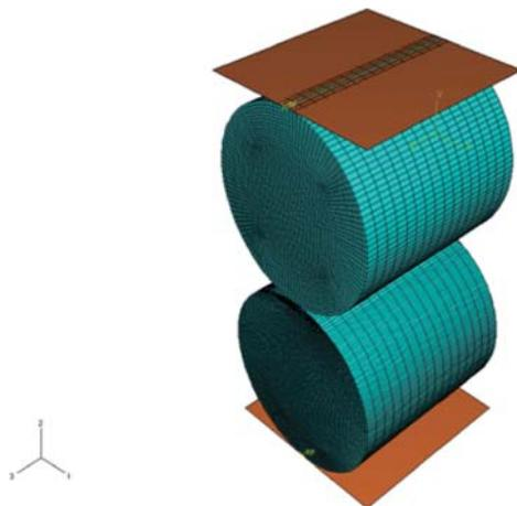
Figure 1. Two identically sized rollers in contact (M 1-00)
