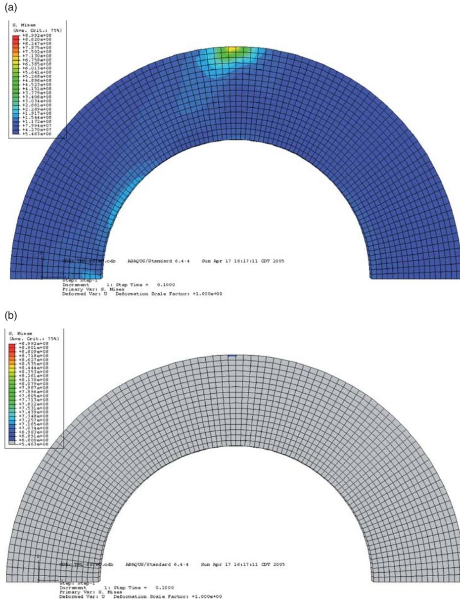
Figure 7. (a) ABAQUS figure of one of two identically sized 60% hollowness rollers in pure rolling contact, (b) ABAQUS figure of one of two identically sized 60% hollowness rollers in pure rolling
