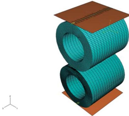
Figure 2. Two identically sized hollow rollers in contact (M 1-60 Two)
