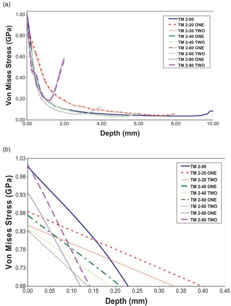
Figure 5. (a) Non-identically sized roller models under combined loading, (b) non-identically sized roller models under combined loading
