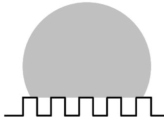
Figure 6. Illustration of the Cassie-Baxter scenario. Air is trapped below the droplet and the solid substrate. The droplet sits upon a patchwork of air and solid surface.
