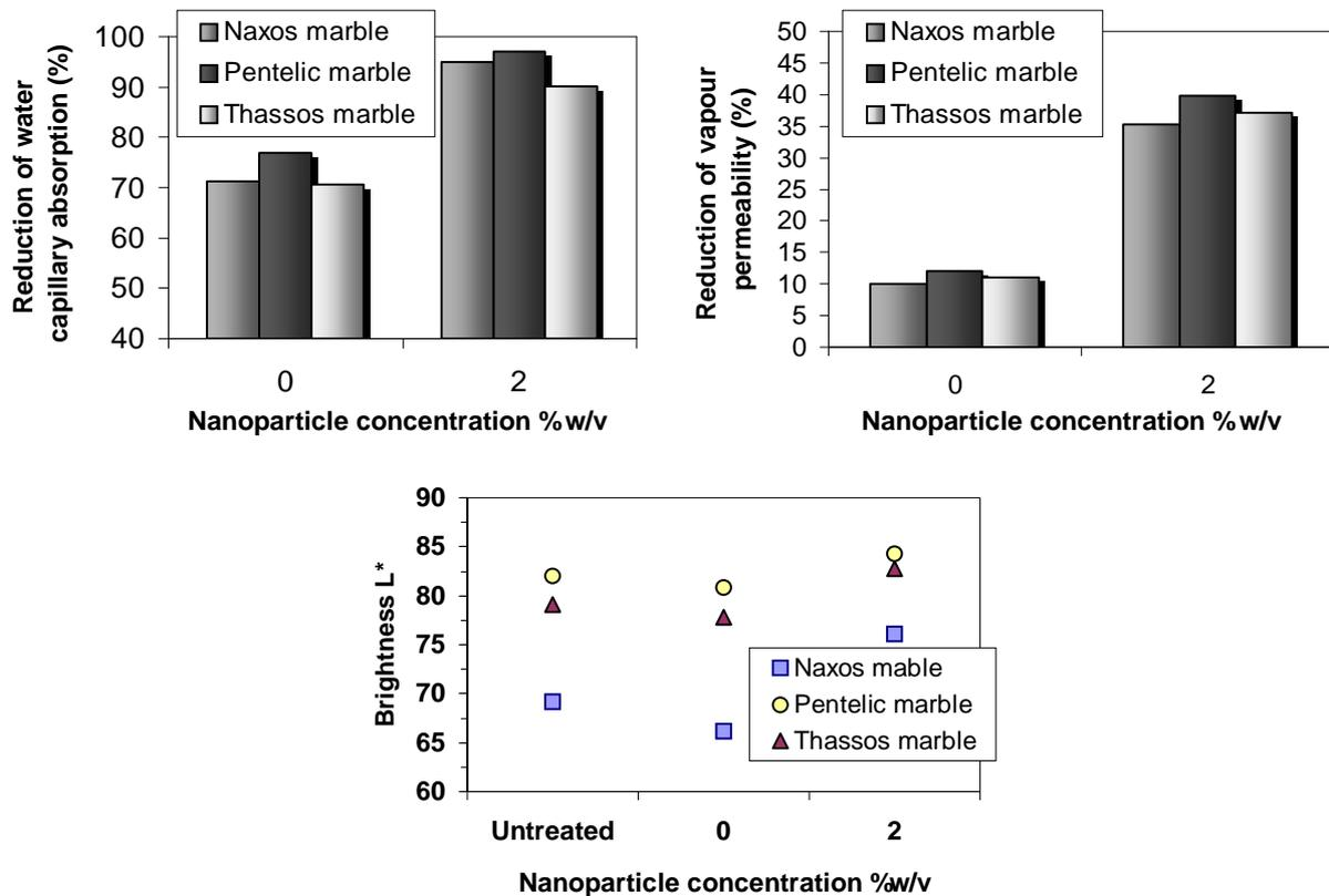
Figure 8. Reduction of water capillary absorption and water vapour permeability for three marbles treated with pure (no particles) siloxane and dispersions of siloxane and particles (2% w/v). Brightness ( $L^*$ ) measurements correspond to untreated marbles and marbles treated with pure (no particles) siloxane and dispersions of siloxane and particles (2% w/v).
