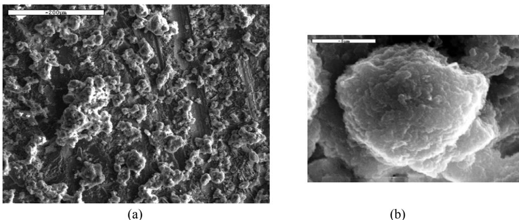
Figure 5. SEM images of Pentelic marble treated with siloxane and 2% w/v nanoparticles.
