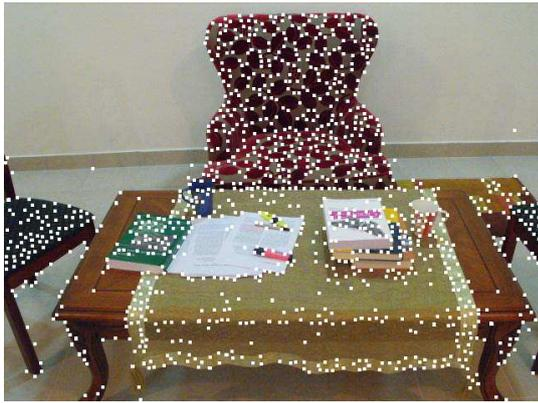
Fig. 1. Feature Extraction using an image of  $640 \times 480$  pixels: 1136 features were detected with inter-corner distance of at least 6 pixels. For inter-corner distances of 9 and 12 pixels, the detected feature points are 698 and 491 respectively.
