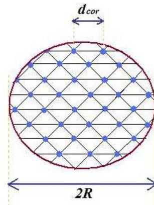
Fig. 5. Triangulated search region in Image 2 to match a feature point from Image 1. The triangles are equilateral with each side =  $d_{cor}$
