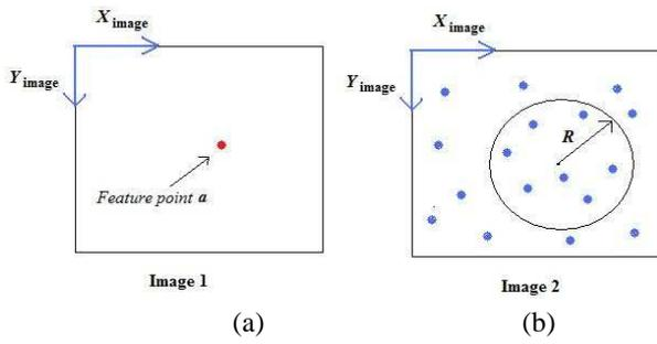
Fig. 4. Image matching: (a) A feature point on the first image (Image 1) to be matched with feature points in the second image (Image 2), (b) The candidate features on the second image are within a circle of radius  $R$ .
